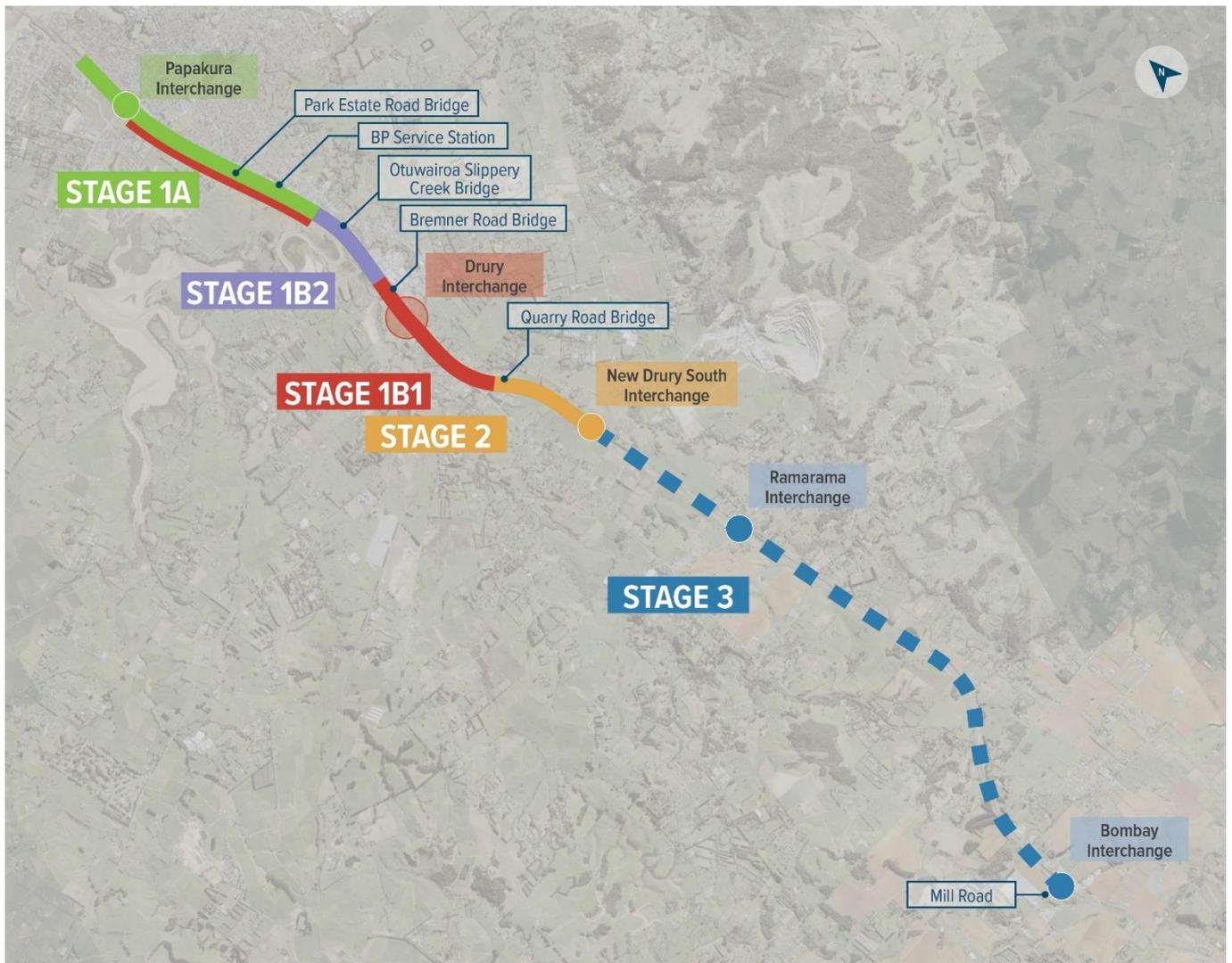
Figure 1-1 Approximate extents of P2B. Focus of this Report is Stage 1B1. Source: Aurecon NZ Ltd
