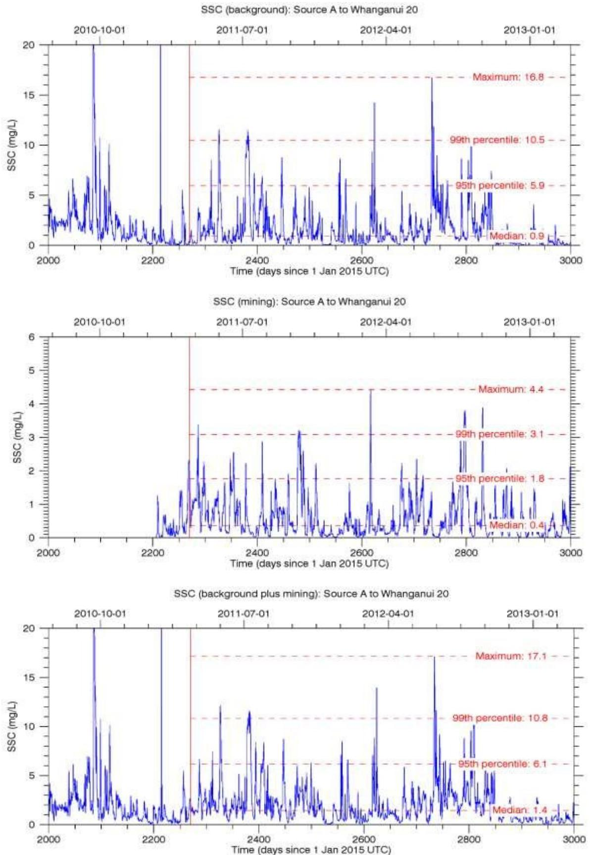
Time series for SSC at 20 km from the mining site when mining at Location A. Note that the changes due to mining are minor and very short-term for the peaks. The difference in the median will have no effect on the planktonic or benthic animals at this site.
