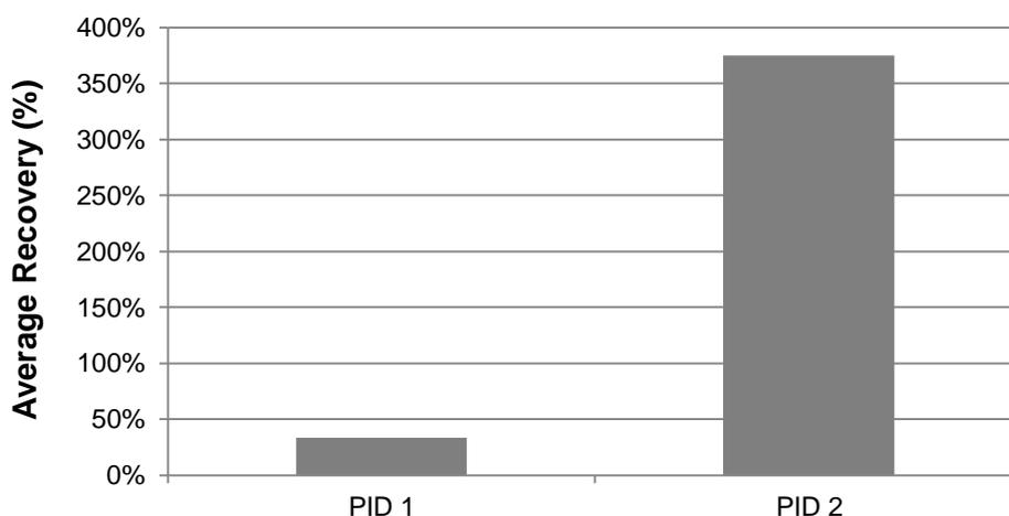
**Figure 4.** Average recovery of methyl bromide in 1-hour TVOC measurements by PID at the monitoring station MS2.
