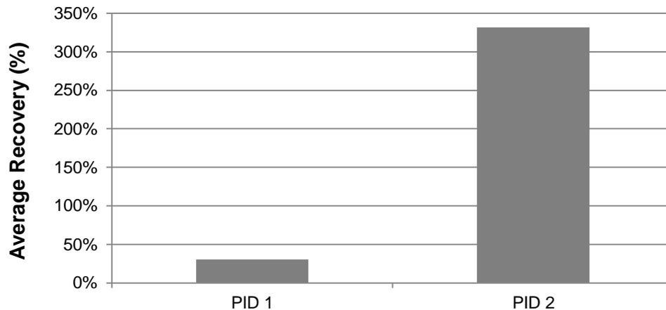
**Figure 4.** Average recovery of methyl bromide in 1-hour TVOC measurements by PID at the monitoring station MS1.
