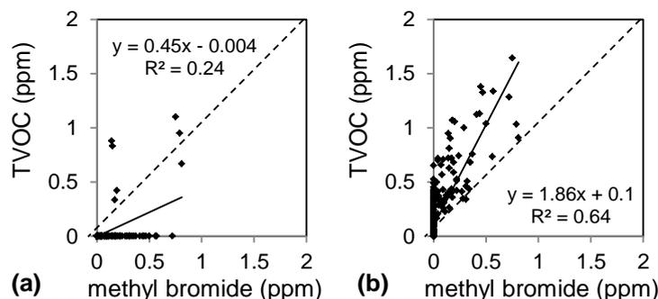
**Figure 4.** Scatter plot of methyl bromide compared to Total Volatile Organic Compounds (TVOC) measured with PID 1 (a) and PID 2 (b) at the monitoring station MS2. The 1:1 line (- -) shows identical concentration.
