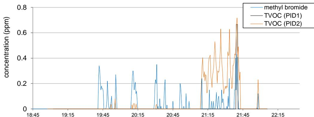
**Figure 2. Time series plot comparison of the concentrations of methyl bromide and Total Volatile Organic Compounds (TVOC) measured with PID 1 and PID 2 at the monitoring station MS1.**
