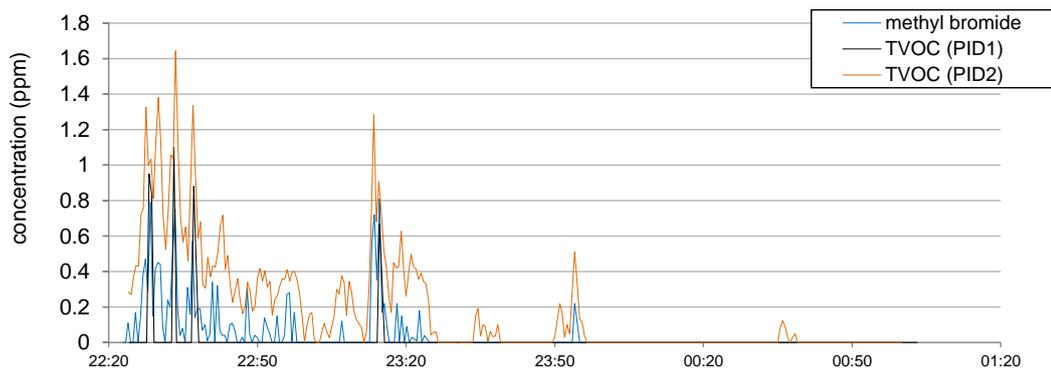
**Figure 5. Time series plot comparison of the concentrations of methyl bromide and Total Volatile Organic Compounds (TVOC) measured with PID 1 and PID 2 at the monitoring station MS2.**
