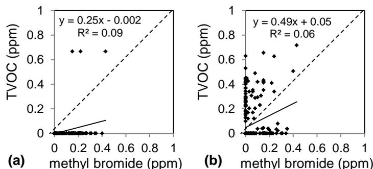
**Figure 3.** Scatter plot of methyl bromide compared to Total Volatile Organic Compounds (TVOC) measured with PID 1 (a) and PID 2 (b) at the monitoring station MS1. The 1:1 line (- -) shows identical concentration.
